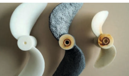
Propeller with (center) and without coating (right) after tribotests in the laboratory.
